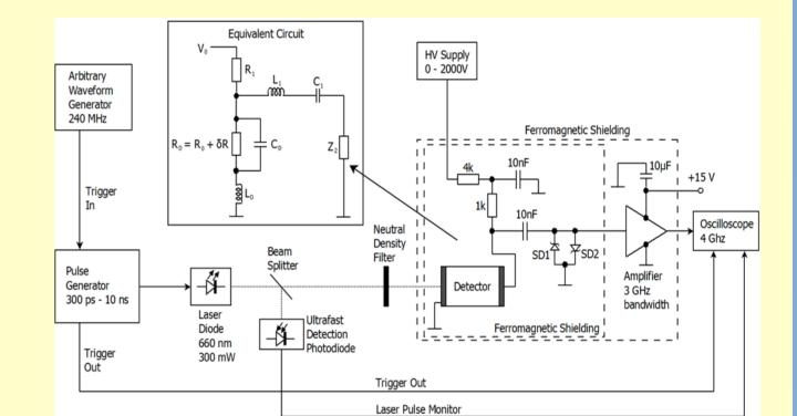
Each measured waveform has to be corrected using deconvolution with the device transfer function Details [4]
