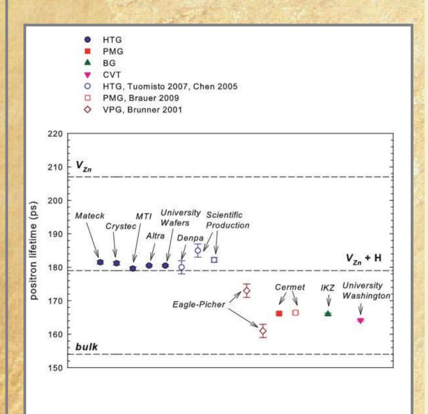
Positron lifetime for crystals grown by several methods and from several vendors. The grow methods are marked by shape of symbols, the producers are marked by arrow. The open symbols represents data from literature.
