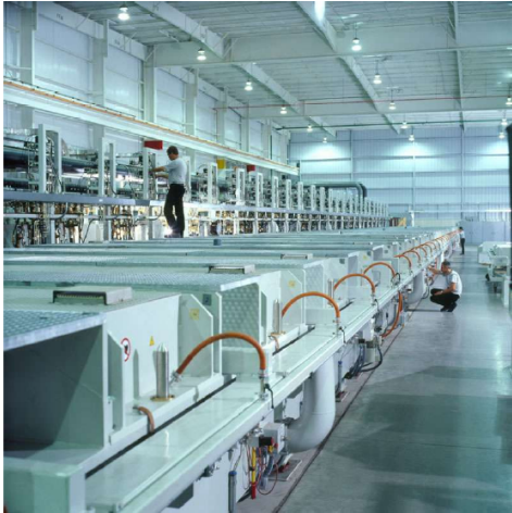
Figure 1: Horizontal inline sputter coater for architectural glass; annual throughput up to 8,000,000 m 2
